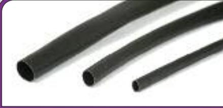
An essential range of lead free, flexible black PVC tubular sleeving, ideal for the protection of wires and harnesses, or for bundling cables together. The PVC sleeving offers excellent chemical resistance to oil, petrol and water, high electrical insulation resistance, and has a wide working temperature range, from -25°C to +105°C.
