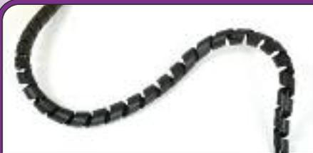
This low density, halogen free, black polythene spiral binding offers a simple and fast method of bundling, binding and protecting cable looms, whilst at the same time allowing wires to be brought from the harness. It has an operating temperature range from -50°C to +85°C
